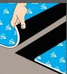
It is important to ensure that all seams between the lengths of underlay butt together so that the overlap sits neatly under the adjoining edge.
