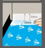
Ensure that the perimeter of the installation is sealed with waterproof tape, running the tape at least 20mm up the walls.
